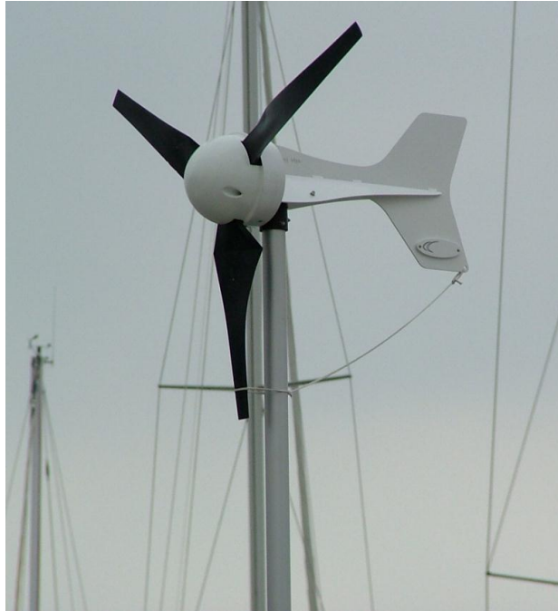
Fig-17: Tethering the rotor blades using the hole on the tail-fin
