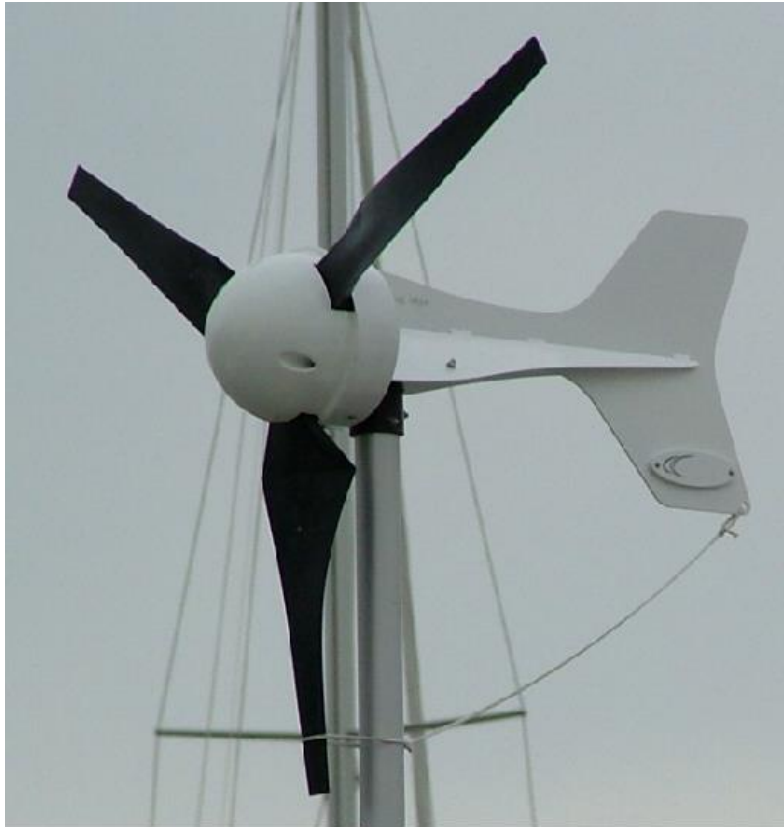
Fig-16: Tethering the rotor blades using the hole on the tail-fin (shown on an LE-300 Turbine)
