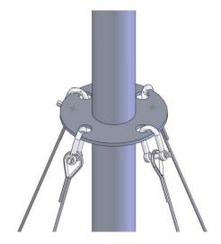
Fig 6: Attach the guy wires to the connection plate
