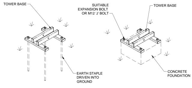
Fig 3: Tower Base Fixing
