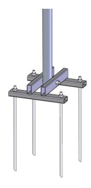
Fig 5: Attached the main tower section to the tower base
