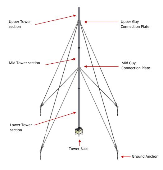
Fig 1: General Guyed Tower Kit Arrangement
