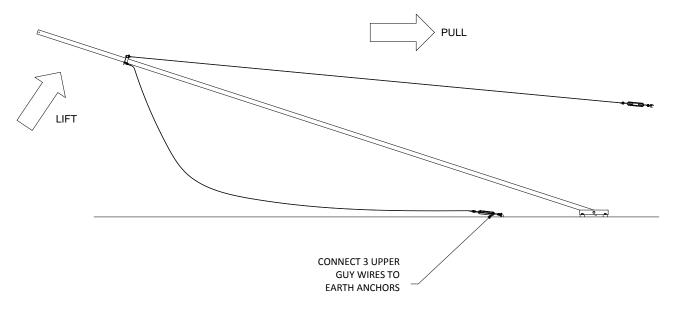
Fig 8: Connect three upper guy wires and hoist the tower
